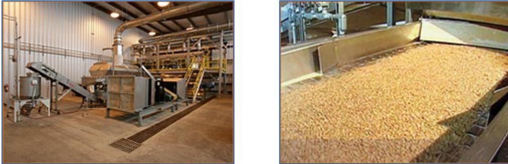
Fig 5. Commercial bran stabilization unit
